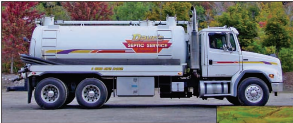
Left, Dave's uses this 4,200-gallon septic pumping truck to service more than 200 restrooms staged over 300 miles. Below, a 24-foot Presidential Luxury restroom trailer is prepped for a post-race party at Hampton State Beach Park.
